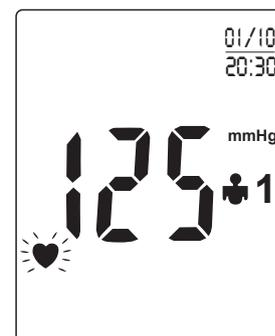
10.4. After measurement is finished the cuff will deflation automatically then the systolic/diastolic blood pressure, pulse rate and blood pressure unit will be displayed and stored. If irregular heartbeat is detected the pulse icon
